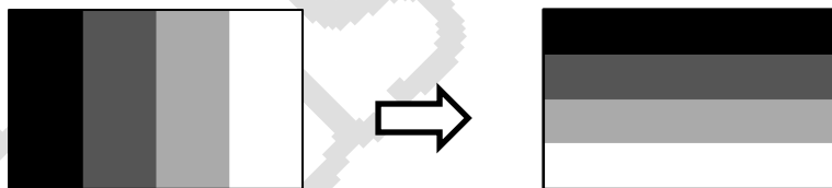
Figure 2 – “Typical” image used for power consumption measurement
