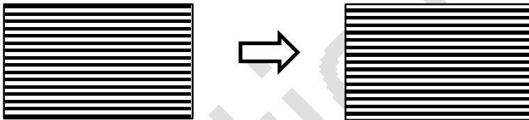
Figure 1 – “Worst case” image used for power consumption measurement
