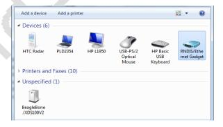
Now your Ethernet connection is enabled. The kit runs a DHCP server so that it is not required to change the network settings of the RNDIS/Ethernet Gadget on the PC. The kit uses the IP address 192.168.7.2 and the PC uses the IP address 192.168.7.1.
