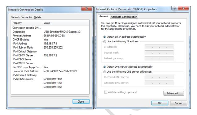
With the Ethernet connection enabled the kit can be accessed via FTP and SSH. The FTP connection does not require a user or a password. The SSH connection uses the same credentials as the serial connection (login "root", password "").
