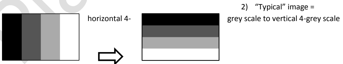
Figure 3 – “Worst case” image used for power consumption measurement
