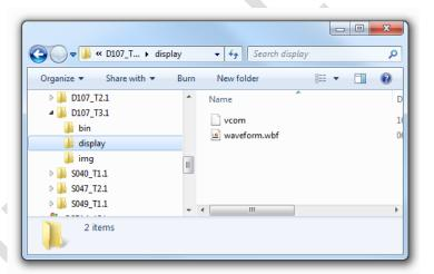
Note: For the 4.0" and 4.9" displays, the waveform file must have the extension .bin.
