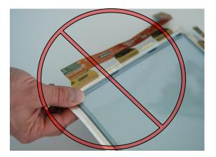
Figure 6 do not hold or bend display at corners
