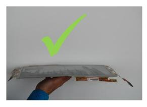
Figure 8 optimum handling (always hold from below)
