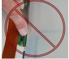
Figure 1 do not apply pressure on chip (IC location)
