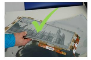
Figure 7 possible position to grip / lift display
