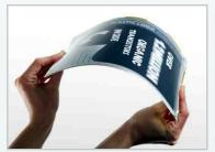
(OTFT) technology provides additional and unique features: Our displays are flexible, extremely robust, glass-free as well as lightweight and ultra-thin. Plastic Logic's displays provide proven lifetimes of over five years and more than 10 million page updates. They are especially suited for applications and products in signage and logistics, mobile electronic devices, smart cards and wearables.
