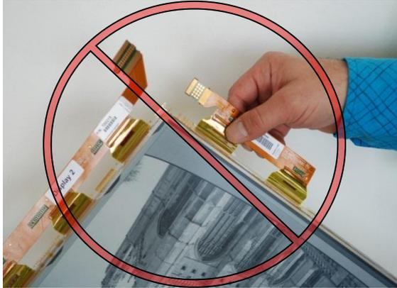
Figure 5 do not hold display on COF/MPWB
