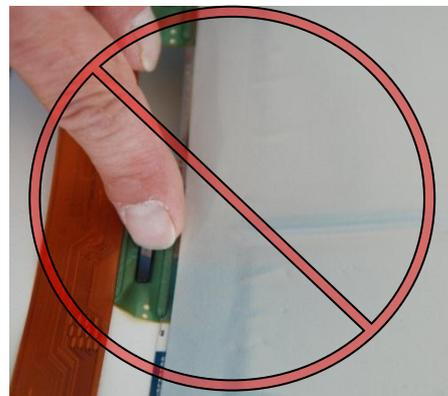
Figure 1 do not apply pressure on chip (IC location)
