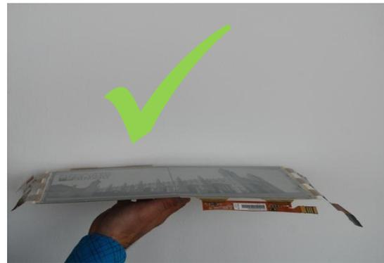
Figure 8 optimum handling (always hold from below)
